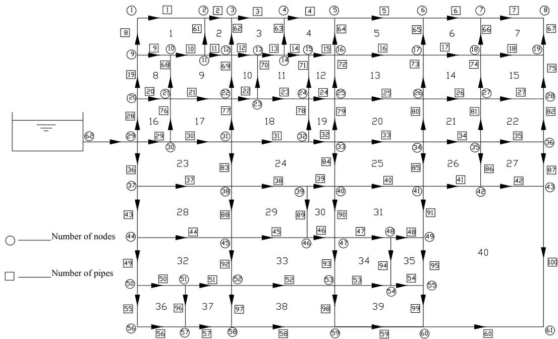
**Figure 1. The networks of a water distribution system**
