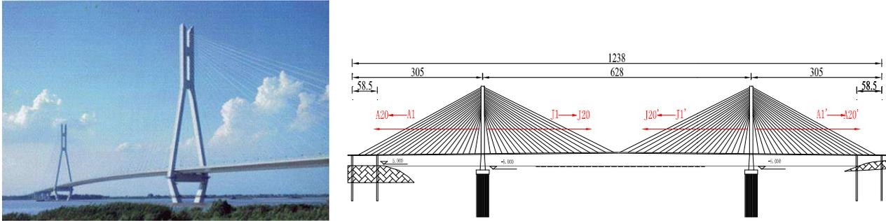
Figure 1 Layout of the bridge
