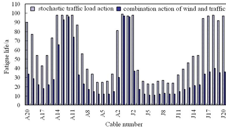
Figure 11 Fatigue reliability life predictions of the cables
