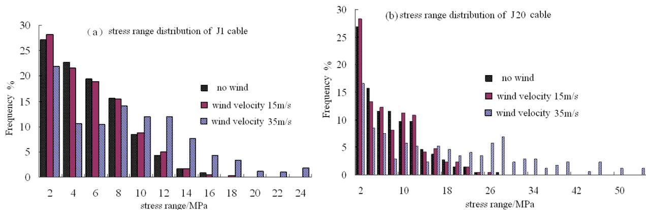
Figure 7 Influence of different wind velocity on cable force under random vehicles
