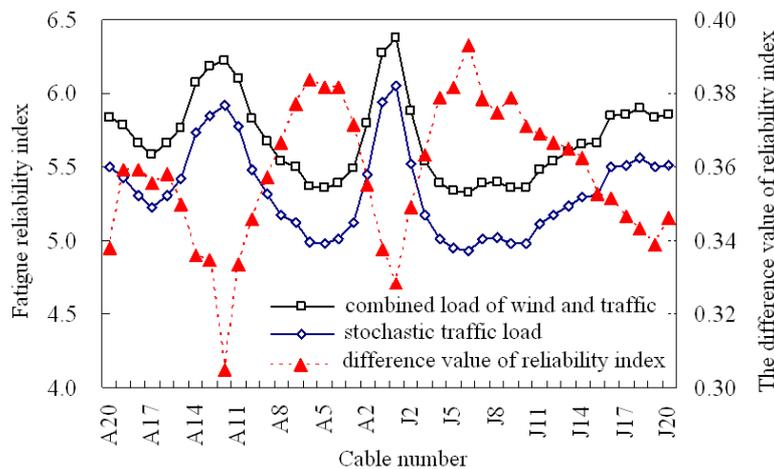
Figure 9 Influence of wind load on cable fatigue reliability
