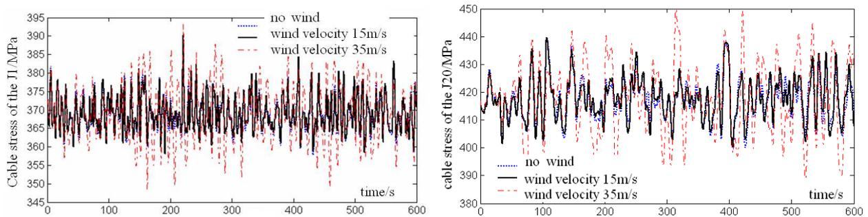
Figure 6 Influence of different wind velocity on cable force under random vehicles
