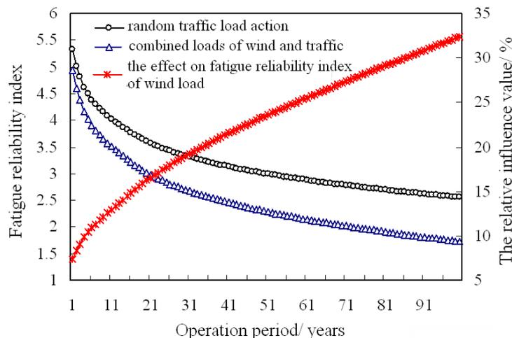
Figure 10 Time-dependent fatigue reliability of the J6 cable
