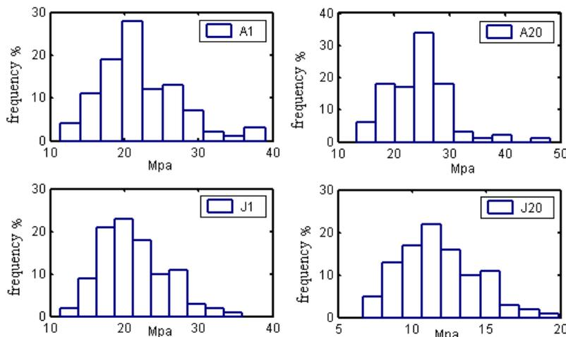
Figure 8 Distribution of cable equivalent stress amplitude
